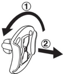
① Rotate the packing locker counter-clockwise through 90 degrees
